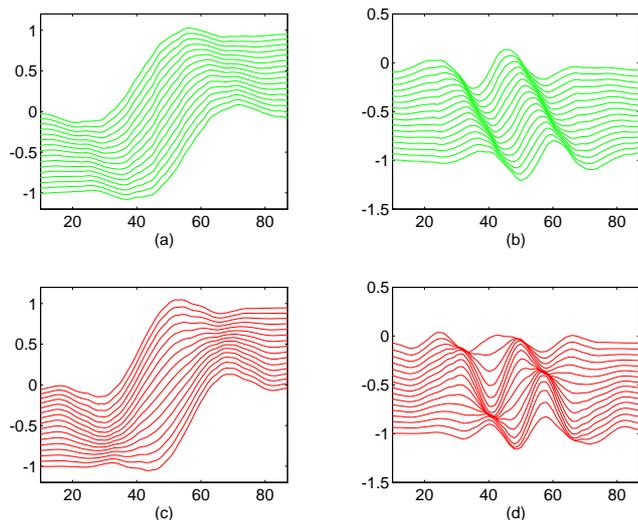
Figure 5: 16 shifted step responses of the complex scaling functions (a) and wavelets (b) at level 4, compared with the same for the real DWT, (c) and (d).
