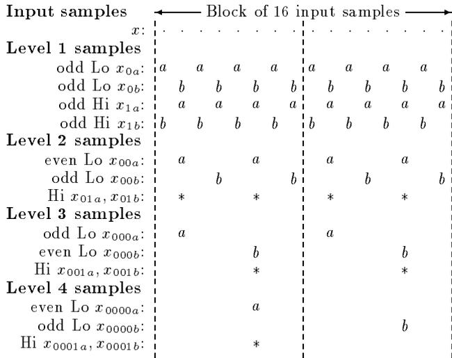
Figure 2: Effective sampling points of odd and even filters in fig. 1, assuming zero phase responses.
