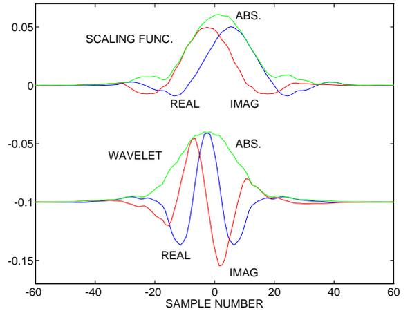
Figure 3: Impulse responses at level 4 of complex scaling function,  $g_{0000b} + j g_{0000a}$ , and wavelet,  $g_{0001b} + j g_{0001a}$ .
