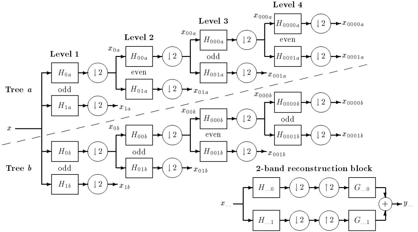
Figure 1: Dual tree of filters for the complex wavelet transform.
