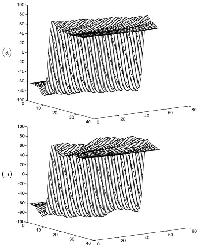
Figure 7: Mesh plot of a gaussian blurred edge, enhanced using the 2-D dual-tree CWT (a), and using the 2-D real DWT (b).
