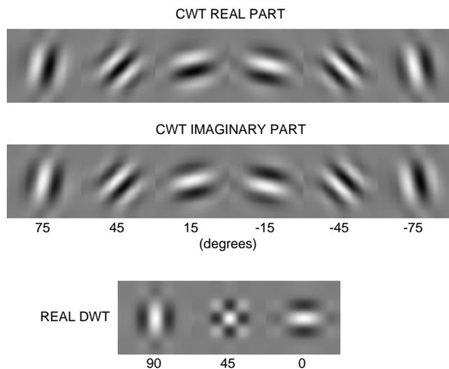
Figure 6: 2-D impulse responses of the complex wavelets at level 4 (6 bands at angles from  $-75^\circ$  to  $+75^\circ$ ), and equivalent responses for a real wavelet transform (3 bands).
